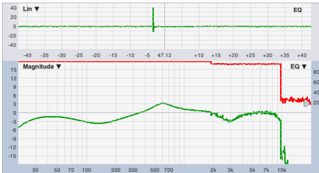
Figure 98: HF coherence loss in the MTW transfer function due to delay mismatch
